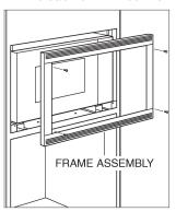
15 Remove the protective covering from the side trim and install one piece per side.
