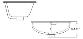
Dimensions shown for location of supplies, waste and mounting clips are suggested. Installation instructions supplied with lavatory. Mounting clips included.
