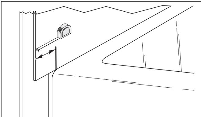
2. Hold the apron strips in place and scribe the angle of the bathtub base onto each piece. Remember, do not cut the finished edge.
