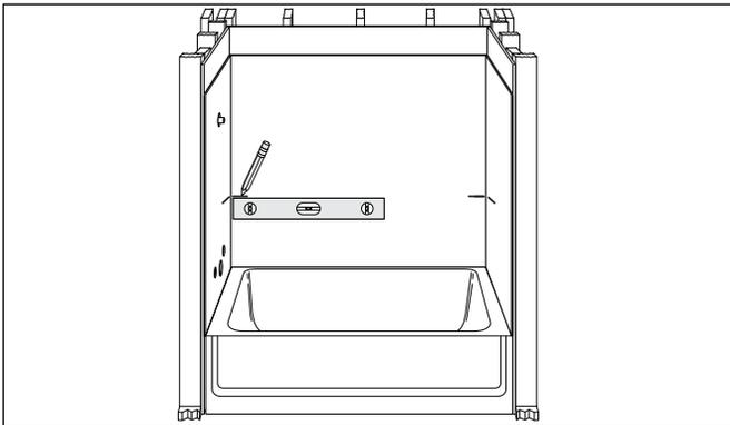
3. Dry fit the soap dish prior to applying clear silicone. The soap dish may require sanding to fit precisely in the corner. The actual angle of the soap dish is slightly greater than 90 degrees to accommodate some adjustment. If necessary, mark and sand the side(s) of the soap dish to achieve a proper fit, using a coarse grit (60 grit) sandpaper.
