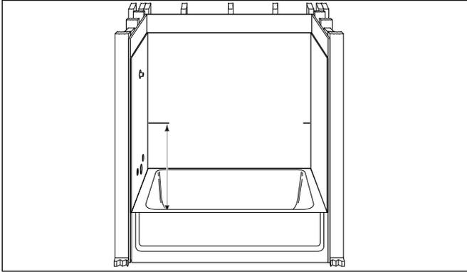
2. After marking the height, draw a 4 inch level line on both walls. These lines will be used to align the top edges of the soap dish.
