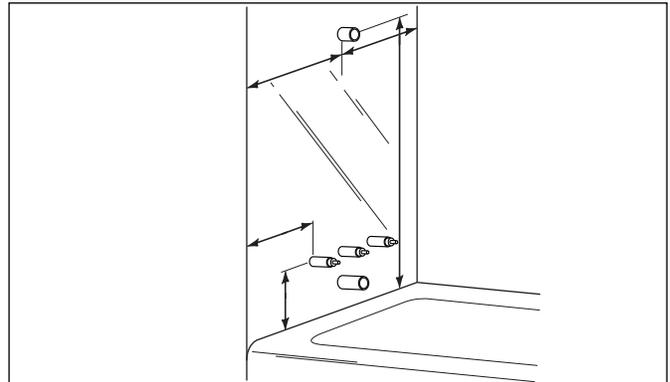
6. Transfer the measurements to the panel.
