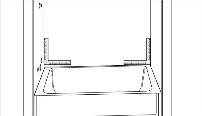
2. If the tub surface is not perpendicular to the wall, use a level and draw a line around the alcove on all three walls. Measure the distance from the line to the top of the tub.
