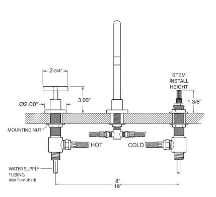
NOTE: Spout and valves install through 1-1/4" diameter holes
