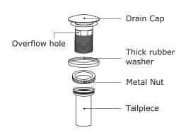
**Step 5 :** From under the drain, insert the thick rubber washer and screw on and tighten the metal nut. Remove excess plumbers' putty.
