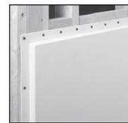
1-1/4" flanges fasten direct-to-studwalls with screws, drywall conceals flanges.
