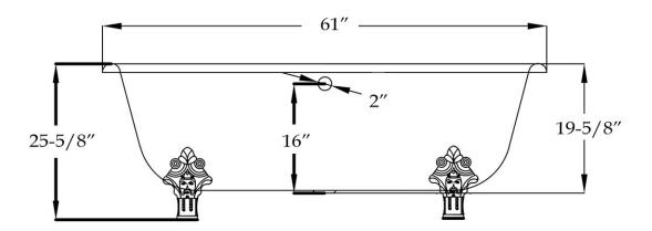
Weight (empty): 319 lbs Weight (filled): 803 lbs Capacity: 58 gal Water depth: 16"
