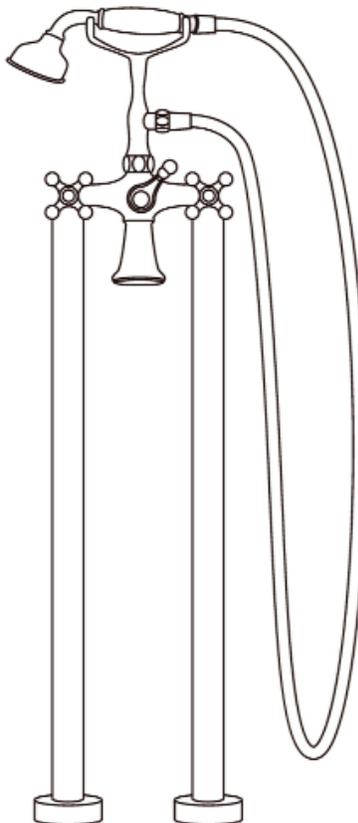
4. Connect the Handshower Hose (6) to both the Handshower and Faucet Body (2). Connect to water supply beneath floor and turn faucet on to test for leaks. Test all 3 handles to ensure water connections for hot and cold are correct and diverter for handshower works properly.
