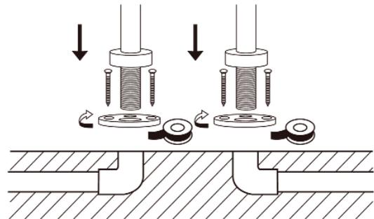
2. Wrap threaded ends of Bath Supplies (2) with teflon tape and thread through Cover Plates (4). Secure Cover Plates (4) to floor with Screws (5) provided. Thread enough through floor to ensure water connections can be done while testing height to ensure proper placement of tub filler over tub rim. Slide Floor Escutcheons (3) down to conceal Cover Plates.
