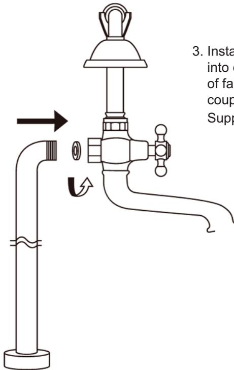
3. Install 2 seal washers into couplings on back of faucet body. Thread couplings to Floor Supplies (2).
